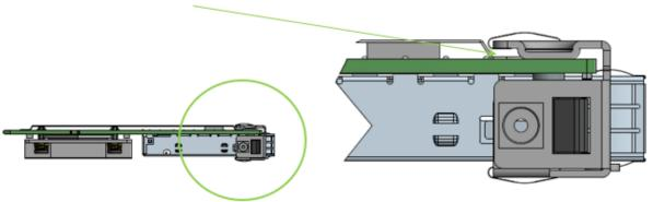
3. Screw on the OCP 3.0 bracket with the supplied screws that came with the new bracket kit. Use the specified torx tool type and apply the specified torque on the screws per bracket form factor.
