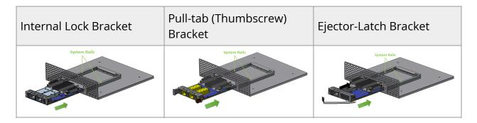
4. Push the card until connectors are in a full mate.
